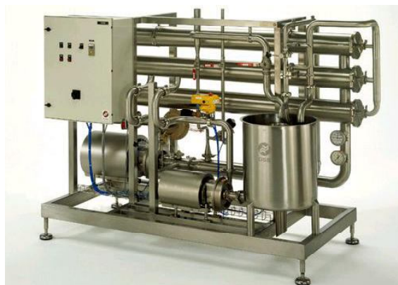
Fig. 12.8 Filter to remove microbiological impurities from cheese brine
