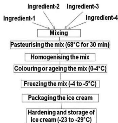
Fig. 3.7 Flow chart for preparation of ice cream
